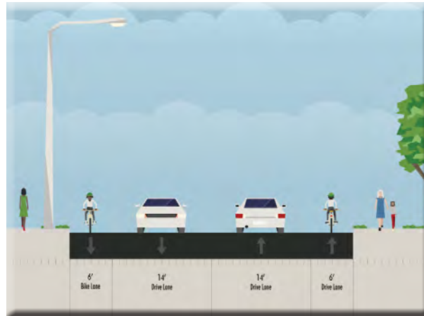
FIG 9-4: Cross-section “F” – Minor (Residential) Collector/60 ft. ROW/40 ft. FOC/with Bike Lanes
