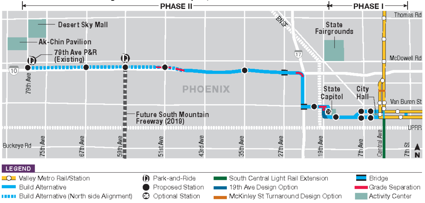
Figure 2.2 – Potential Capital/I-10 West LRT Extension Route
