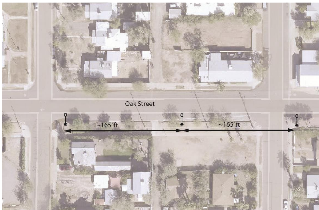
Figure 2 - Typical Light Pole Spacing
