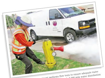
The Water Services Department performs flow tests to ensure adequate water pressure for fire protection throughout the nearly 7,000 mile water distribution system.
