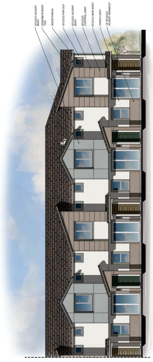
FRONT ELEVATION - 9 PLEX - 4 UNIT MODULE 3/16" = 1'-0"
