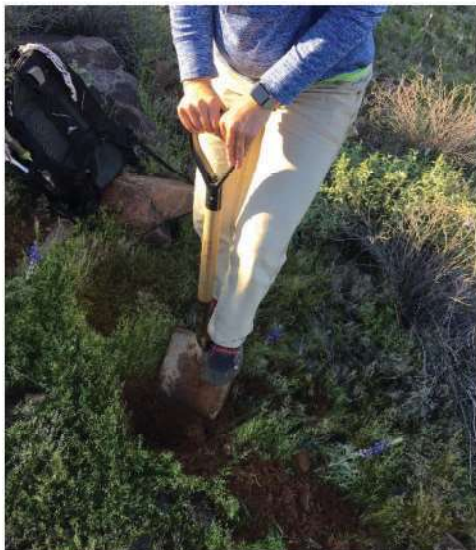
PHOTO 5: Sample location dug to depth prior to sample collection
