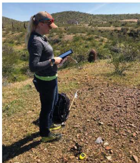
PHOTO 4: Recording GPS coordinates of sample location in Fulcrum application
