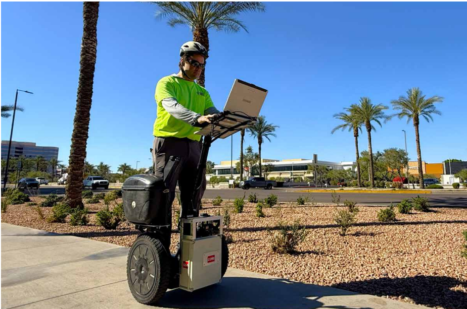
For ADA inventory assessments, this custom-built Segway travels along sidewalks across the city to capture data on slope, cross slope, sidewalk heaves and other deformities.
