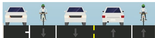
PROPOSED Travel Lanes on 65th PI / Montreal PI from 66th St to 68th St
