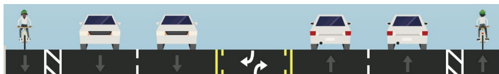
Proposed Travel Lanes (Typical Cross Section, existing turn lanes will be preserved)
