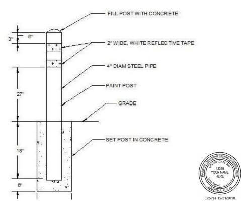
IMPACT SCENARIO: The expected vehicle traffic for (Facility Name) is (Light-Duty; Medium-Duty; Heavy-Duty), for which the vehicle impact protection detail provides the required protection from impact for.
