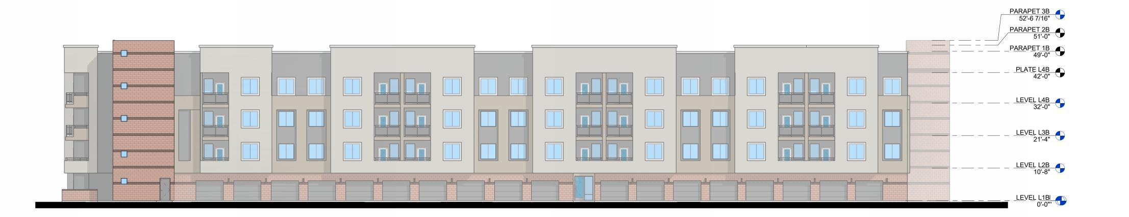
9 BLDG 2&3 - SOUTH ELEVATION 0' | 16' | 32' | SCALE: 1/16" = 1'-0"
