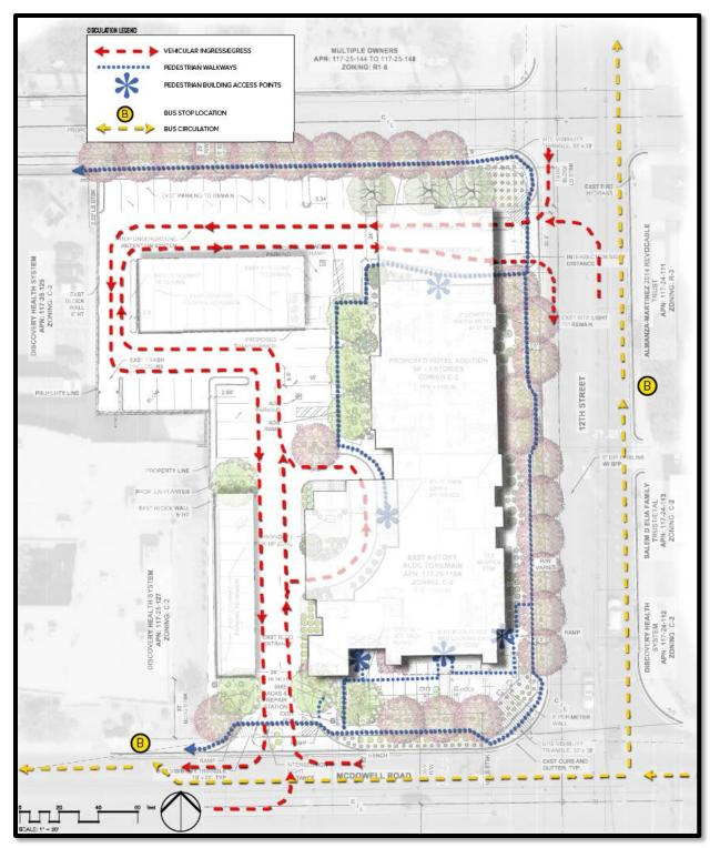
Figure 6 Vehicular Circulation Plan
