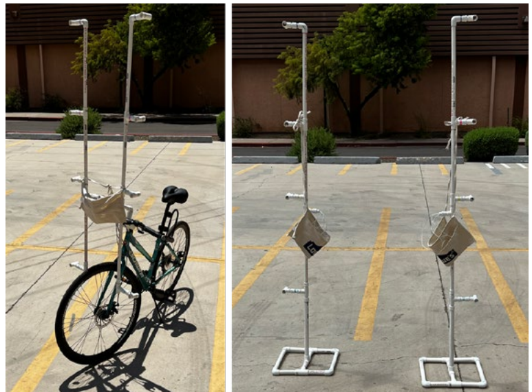
Fig. 3: High-precision vertical air temperature gradient
