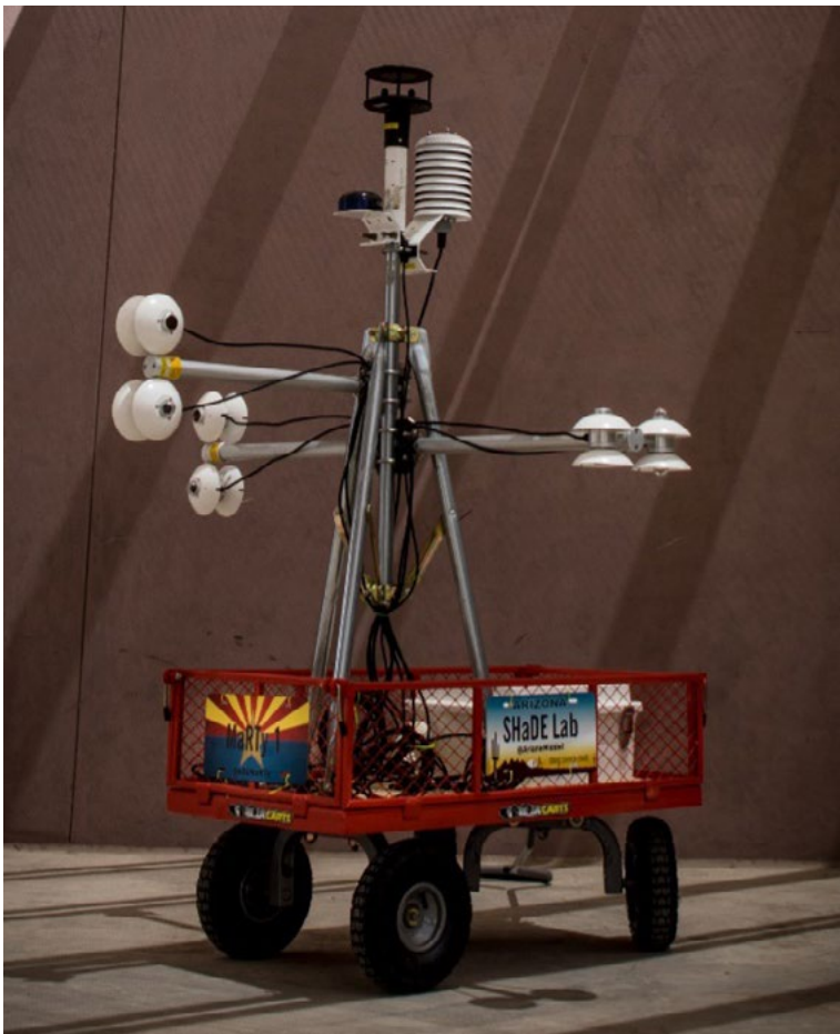
Figure 2: MaRTy, the biometeorological weather station.
