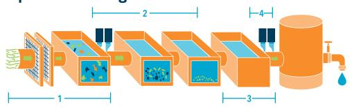
Screening and Presedimentation - Large particles such as plant matter debris, and other materials commonly found in river water are removed by screens or settle to the bottom of the presedimentation basin.
