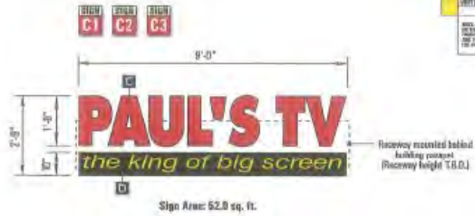
NORTH, WEST & SOUTH ELEVATIONS SETS Scale: 3/8" = 1'-0" Proposed "Paul's TV" illuminated channel letters
