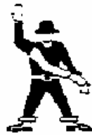
RELEASE SLING LOAD Left arm down away from body. Right arm across left arm in a slashing movement from above
