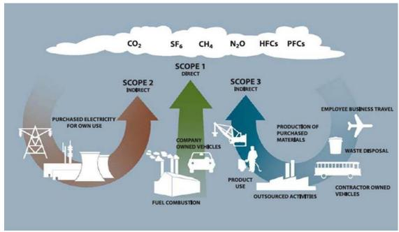
Figure 1: Overview of LGOP Scopes and Emissions Sources.
