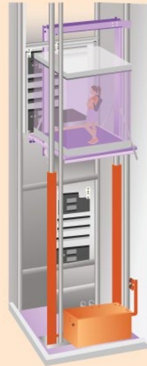
Hydraulic MRL - Machine Room-Less
