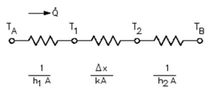
$$\tilde{Q} = \frac{T_A - T_B}{1/h_1 A + \Delta x/kA + 1/h_2 A}$$
