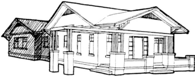
Subordinate rear addition using similar shape, window proportions, and roof form. Note the smaller transitional element between the historic house and new addition.
