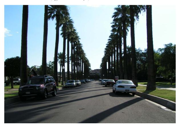
**Figure 27. Portland Street between 3rd and 5th avenues.** This streetscape has original features such as high curbs, grassy planting strips with mature palms, period light fixtures, and standard setbacks and architectural styles. Photograph by Vincent Murray.
