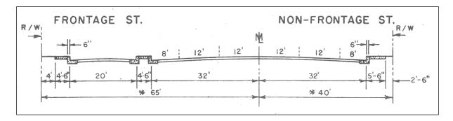
**Figure 23. Frontage Street with Traffic Separation Strip.** From *Inventory and Appraisal of Street Deficiencies.*
