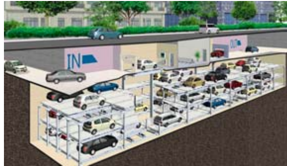
Example of an automated parking storage and retrieval system. Credit: Sumitomo Heavy Industries, Ltd.
