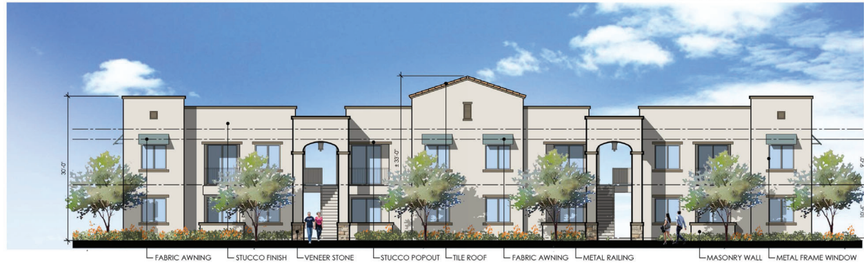
FRONT ELEVATION (REAR ELEVATION SIMILAR) BUILDING TYPE 2
