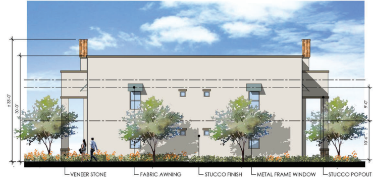
RIGHT SIDE ELEVATION
