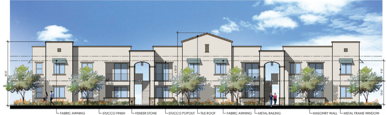
FRONT ELEVATION (REAR ELEVATION SIMILAR) BUILDING TYPE 1
