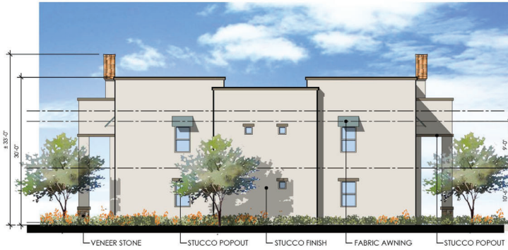
LEFT SIDE ELEVATION
