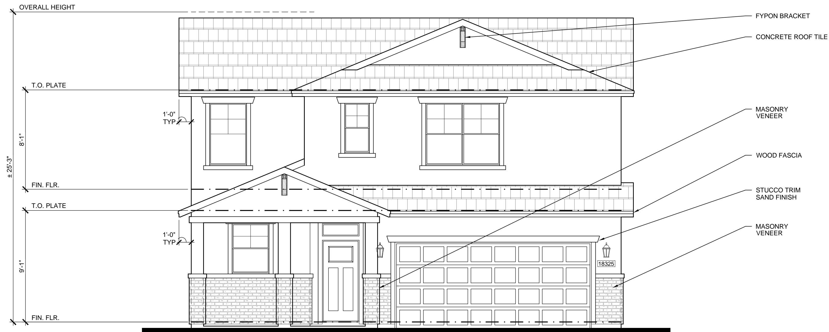
FRONT ELEVATION ELEVATION O 1/4" = 1'-0"
