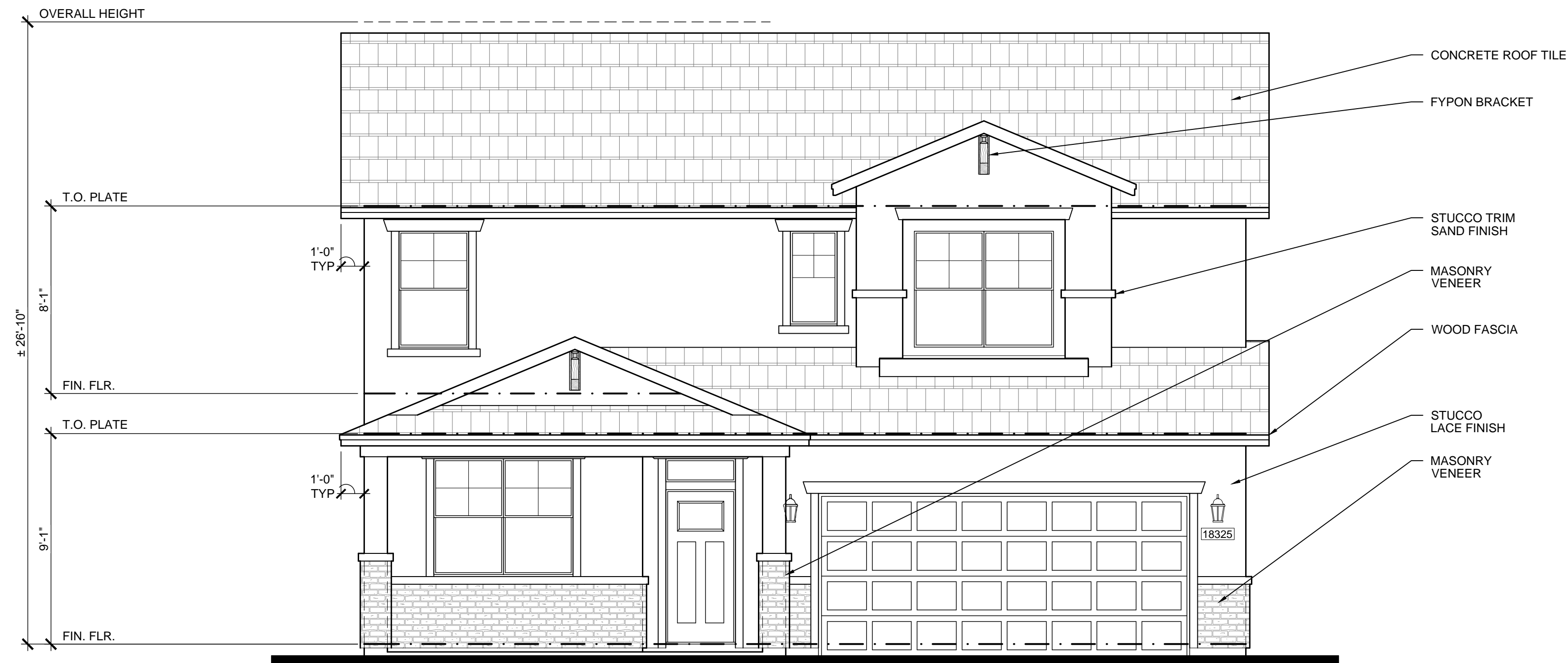
FRONT ELEVATION ELEVATION O 1/4" = 1'-0"
