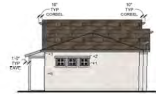
Left Elevation Elevation A - Cottage 1/8" = 1'-0"
