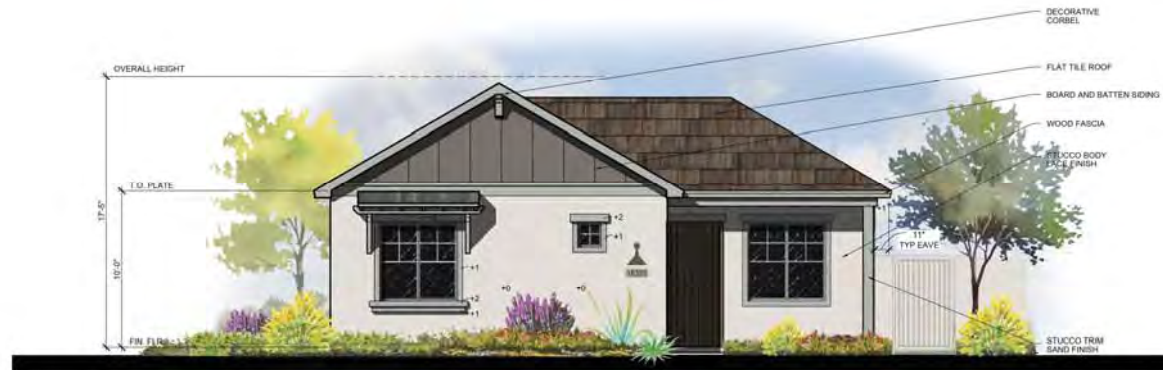
Front Elevation Elevation A - Cottage 1/4" = 1'-0"
