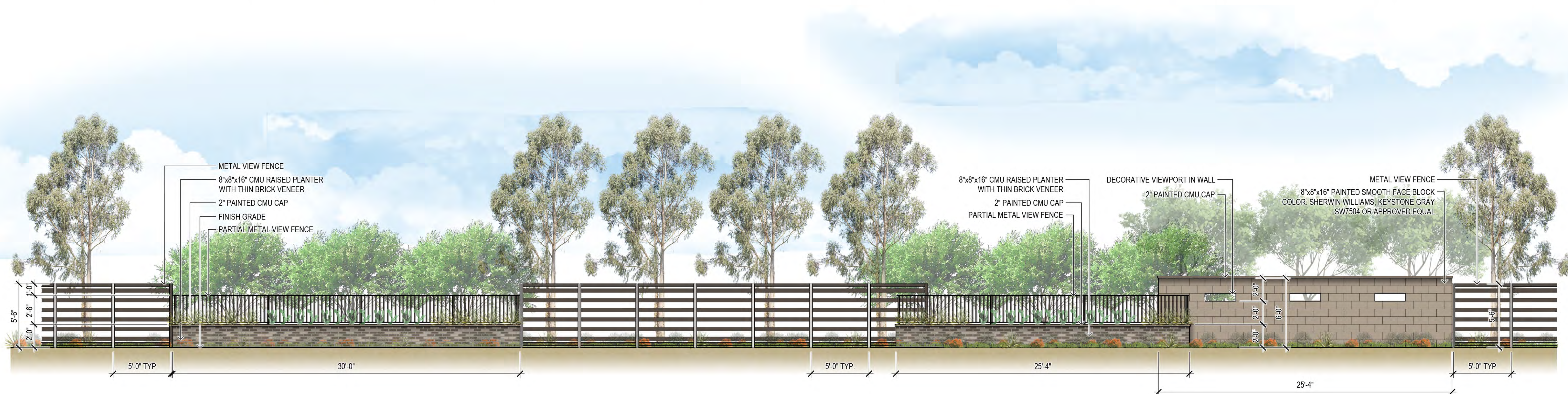
2 55th Avenue Wall Condition (Elevation) SCALE: 1/4"=1'-0"
