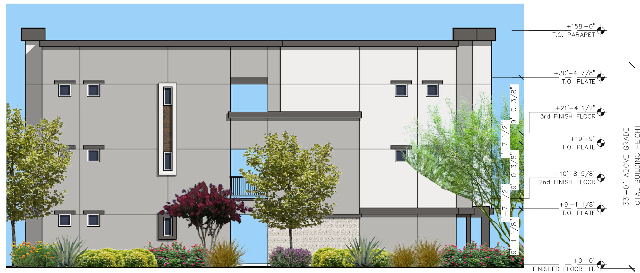
BUILDING TYPE 2 - SIDE ELEVATION
