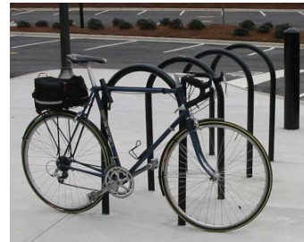
Inverted-U bicycle rack, where both ends of the "U" reach the ground.
