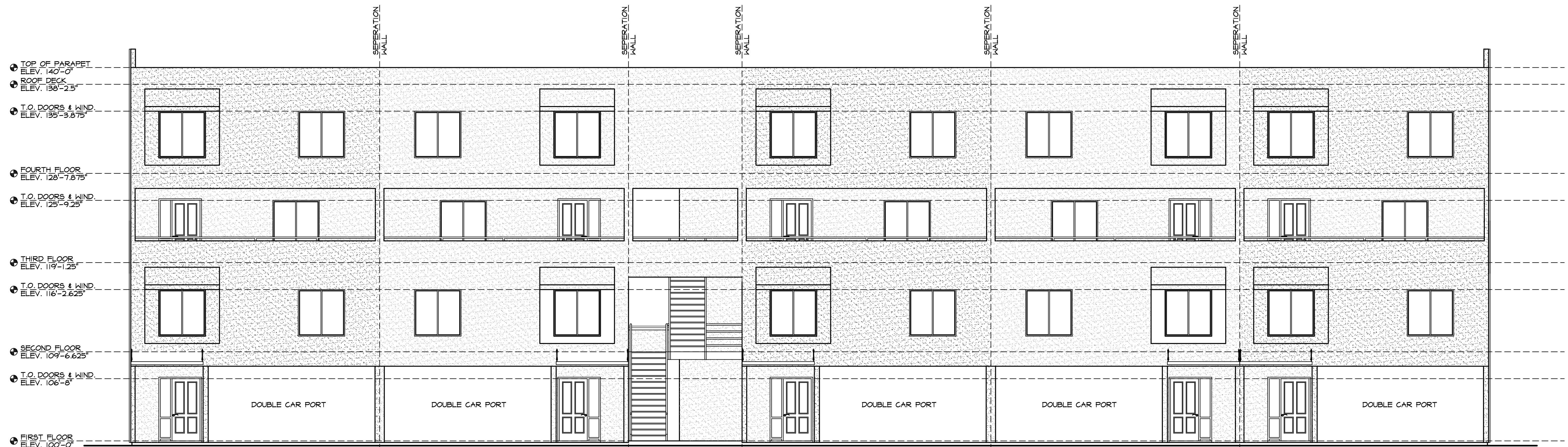
A FRONT ELEVATION (5 UNITS) SCALE: 3/16" = 1'-0"
