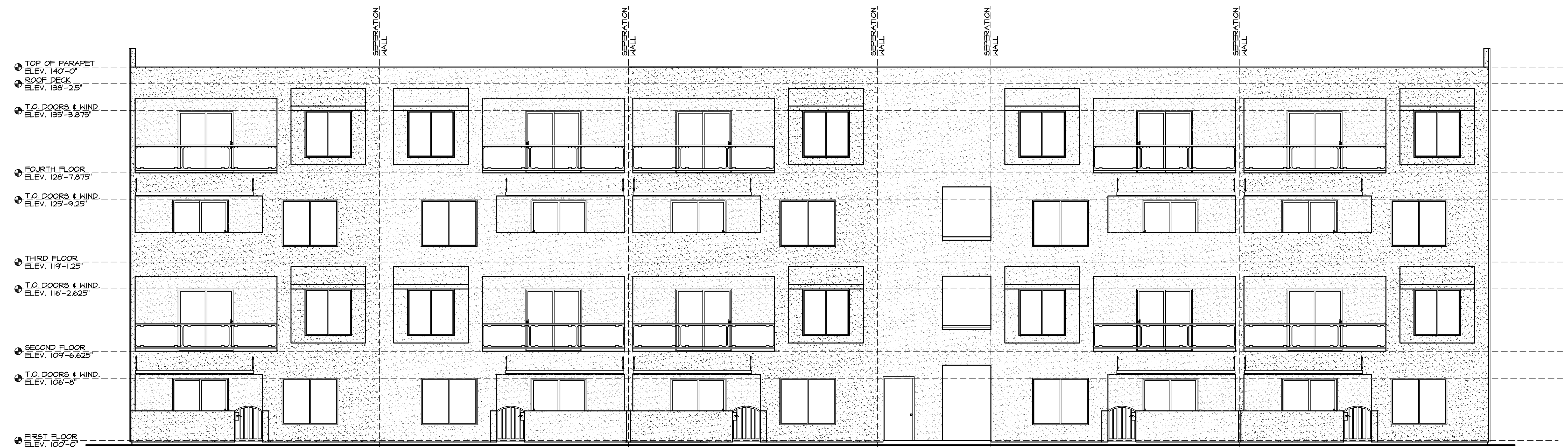
B REAR ELEVATION (5 UNITS) SCALE: 3/16" = 1'-0"
