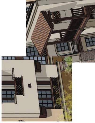
DECORATIVE BALCONY ELEMENTS WITH RAFTER BASE TAIL PROFILES & BRICK OR IRON METAL RAILING
