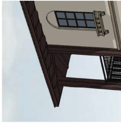
TERRA COTTA TILE ROOFING (3:12 PITCHED & 4'-0" HT.) & TRIM PROFILE; EAVE OVERHANG WITH EXPOSED RAFTER TAILS
