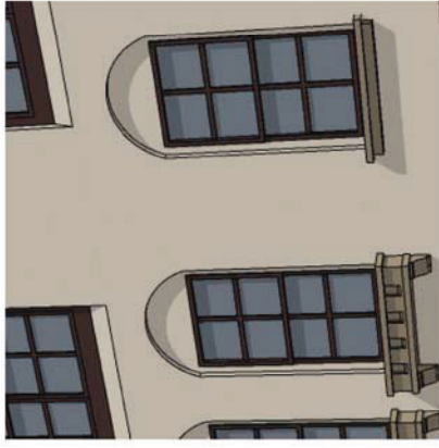
ARCH ABOVE DOOR OR WINDOW WITH STONE BASE WITH DIFFERENT PROFILES OR RECESSED ANGLE BASE
