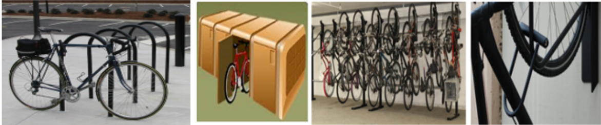
Inverted-U bicycle rack, where both ends of the "U" reach the ground.
