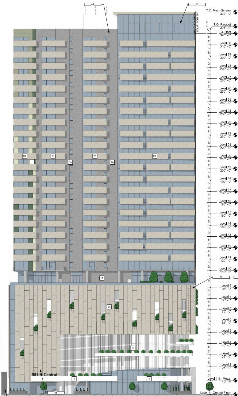
2 EXTERIOR ELEVATION - WEST (N CENTRAL) SCALE 1/16" = 1'-0"
