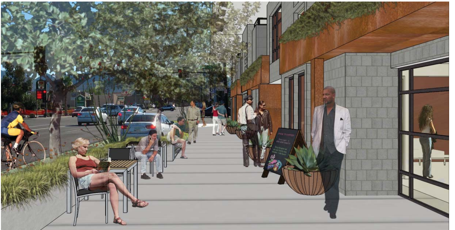
Concept design for re-purposed commercial development at the northwest corner of North 32nd Street and Shea Boulevard. This concept includes an on-street bike lane, two north and two south vehicular travel lanes (no center turn lane), wide sidewalks and mixed use retail/residential development along the street.
