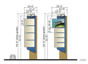
**1.3** - Project Parcel ID Pylon Scale: 1"=24'-0" **1.3** - Project Parcel ID Pylon w/Electronics Scale: 1"=24'-0"
