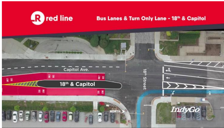
Transit Spot Improvements
