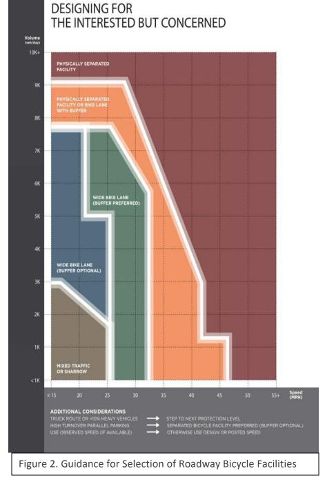
On roadway sections with higher traffic volume and speed, proposed improvements included buffered and protected bicycle lanes, providing greater separation from traffic in the adjacent travel lane. To create buffered and protected lanes, existing travel lanes will need to be narrowed, helping to reduce vehicle speed, an added benefit to both bicyclists and pedestrians.
