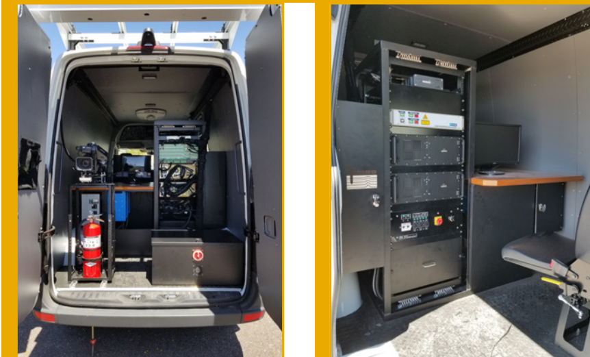
ARAN 9000 Van (interior showing equipment)
