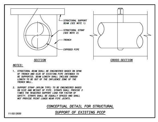
Figure 7. Conceptual Detail for Structural Support of PCCP.
