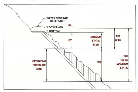
Figure 4. Typical Major Water Pressure Zone Configuration (rounded to the nearest 10 psi).
