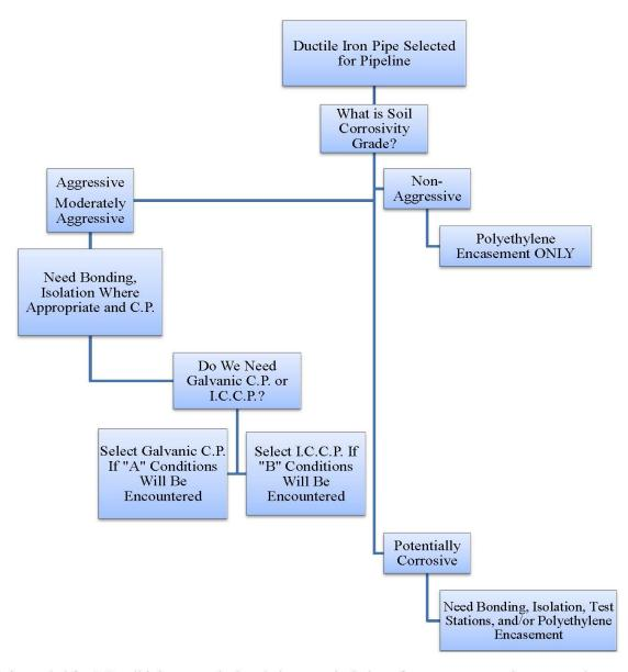
If C.P. is needed for DIP, all joints must be bonded, proper isolation of structures not to be protected must occur, and test stations will be necessary.
