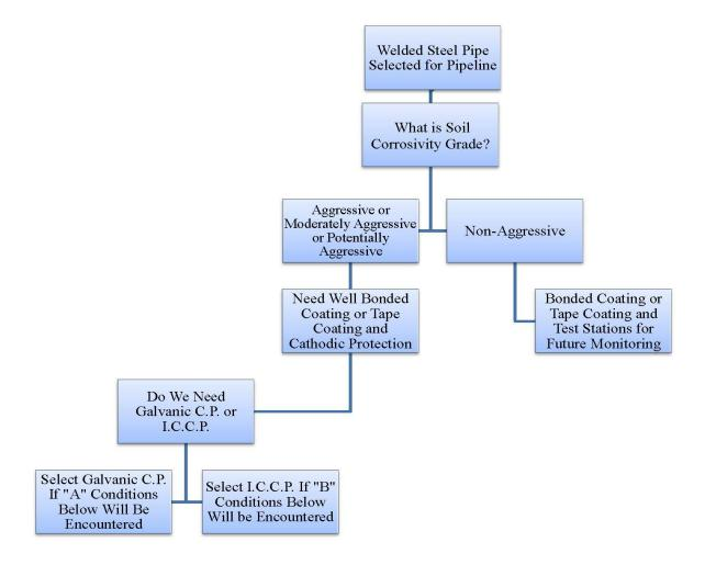
In all cases where C.P. is provided, proper electrical isolation of structures not to be protected and good electrical continuity along the pipeline to be protected must be ensured.
