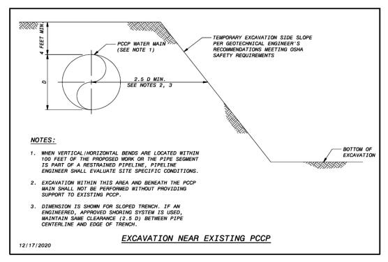
Figure 6. Excavations Near PCCP.
