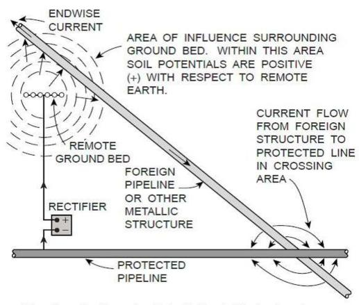
Figure 1 Stray Current Interference from Peabody's Control of Pipeline Corrosion
