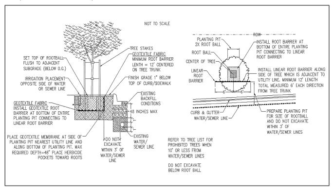
Figure 3. Plant Root Barrier Detail.
